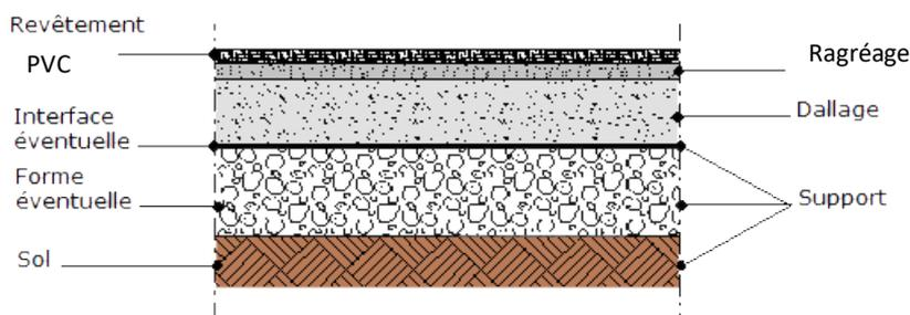
Figure 7 Composition dalle béton
